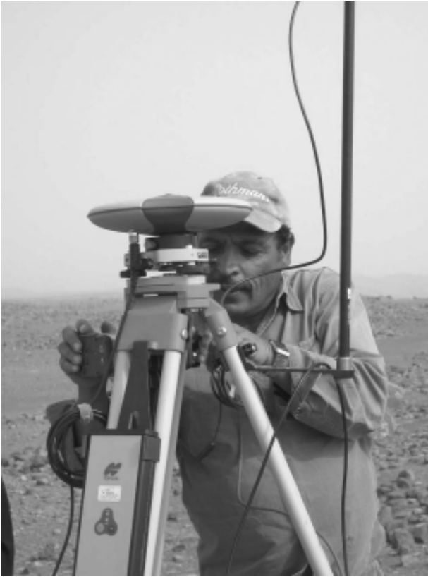
Abdul Basset Noaman sets up the differential GPS base station used of the Masna'at Maryah map.
